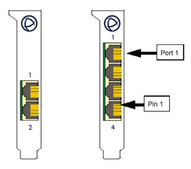
The RJ45 connector has a 10-pin configuration. If you require an 8-pin connector configuration, use the pinouts in the RJ45 8-pin column. The connector pinout for each RJ45 socket fitted to the SPEED LE Express cards is as follows;
